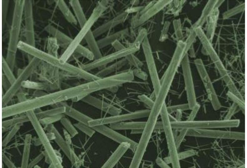
There is a big difference between SI-TUFF™ fiber and microfiber, and the dispersion techniques can be quite different as well. The dimensions of each are:
