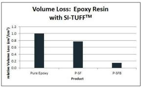
All products 3% loading in Epoxy. Struers ABRAPOL polisher with 320 grit SiC Sandpaper, 100 N force, 300 rpm, 90 seconds, repeat in triplicate.
